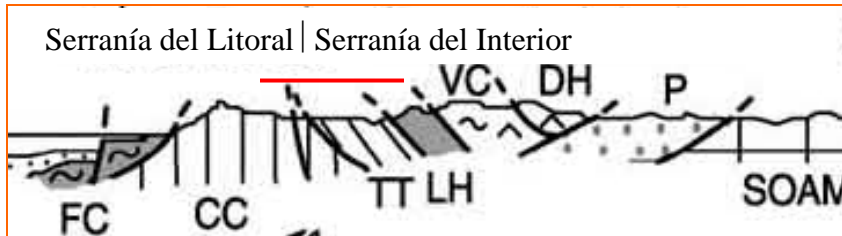
Fig. 7. Rough geological cross-section at 67W. Red line: section covered by this leg. CC: Ávila and Caracas nappe. TT: Caucagua – El Tinaco nappe. LH: Loma de Hierro nappe. From GIUNTA et al. (2000).
